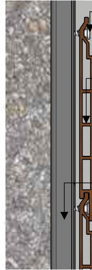
RESCPS25 Resysta Stainless Steel Screw RESCPH120612 Siding Board RESSHTC10 Aluminum Hat Channel SECTION RESYSTA HORIZONTAL SIDING
