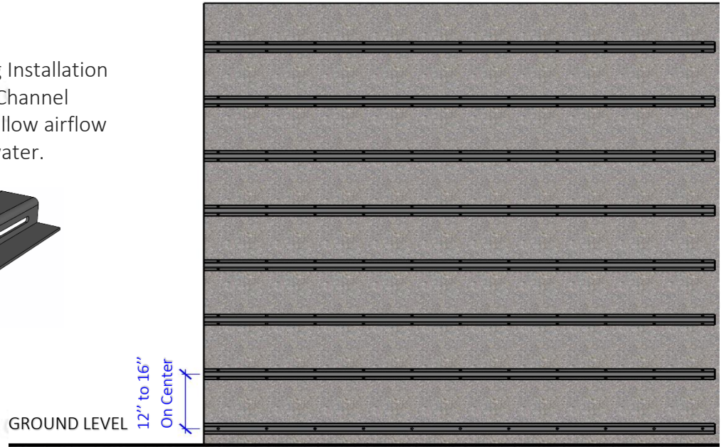
FRONT ELEVATION VERTICAL SIDING / HORIZONTAL BATTENS
